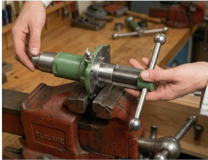
Fig. II Refacing Water Seal Face with Churchill Tool No. 6300 and Bush S.126.
