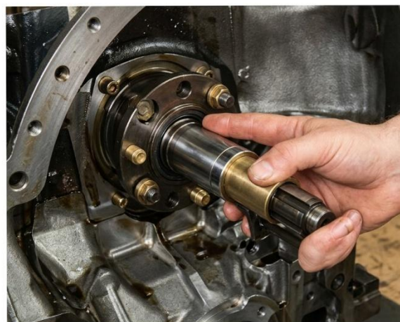
Fig. 29 Assembling Front Cover, utilising Churchill Tool No. 20SM. 47 to protect Seal Face.
